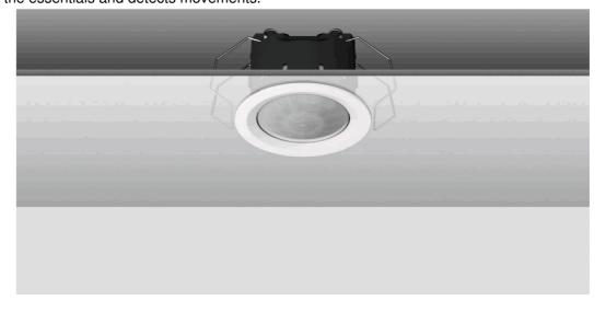
The detector has a PIR sensor and uses it to accurately detect movements through 360 degrees independent of brightness. The sensor works reliably both tangentially (3 m) and radially (2.5 m): it detects movements across the detection area just as accurately as people moving towards or away from the sensor.
