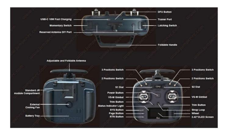
**Note:** To prevent T14 from entering DFU mode during charging and to reduce the probability of firmware loss during charging, T14 is equipped with a separate Boot button. To enter DFU mode, shut down the radio, press and hold the Boot button, and then connect the USB cable.
