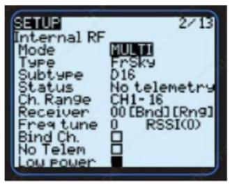
• **Frequency** tuning. Certain protocols require tuning for optimal performance. In some cases, tuning is required for the protocol to bind. Frequency Tuning is specific to each MULTI-Module and is due to very small variations in the RF components.
