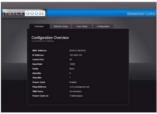
The Overview Tab displays the current settings of the unit and the MAC ad-dress. This page is useful for retrieving all the information you may need to set up the iP PD1-4 on your network. If you have DHCP enabled, the IP address your router/DHCP server assigned can be viewed here.
