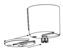
Make sure to check the tray frequently, especially after grinding, to ensure optimal function of this part and avoid material accessing the Jtube carousel part of the machine.
