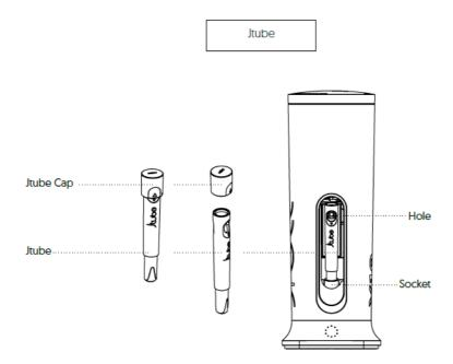
The Jtubes are designed for standard King-Size paper cones, which can be obtained from various suppliers and brands. When placing the Jtubes in the Jroll X10, make sure the hole is facing you and gently place the Jtube into the Socket. Embedded magnets at the bottom of the Jtube assist with proper seating of the Jtube.
