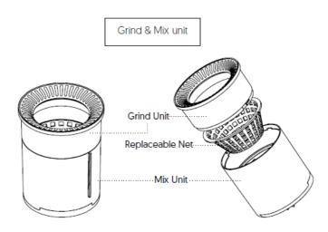
When inserting the Grind & Mix unit into the machine, make sure that the Lip is pointing towards to you (see image below on the left) and aligns with the Groove inside the Jroll X10 and the small printed triangle on the device (see image below on the right). Do not force the unit inside. If aligned, as described above the Grind & Mix unit will slot in smoothly. Inserting the unit incorrectly can cause serious damage!
