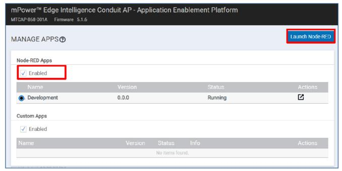
Connect to the Node-RED interface with the same identifiers used to connect to the configuration page of the Gateway:
