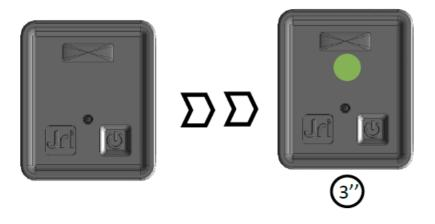
Once the battery is inserted, the device is activated after three seconds. Once activated, the Nova SPY automatically declares itself in MySirius if it is in contact with a Link. It starts measuring and transmitting its readings to MySirius as it goes along, then flashes regularly according to its status.
