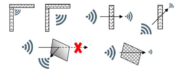
A solid metal wall will not allow radio transmission. A perforated metal wall will allow waves to pass while attenuating them.
