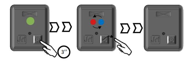
Once the device has been declared in MySirius, the touch button shutdown function is deactivated to prevent "accidental" shutdowns when handling the device. However, this option can always be re-enabled in MySirius to switch off the Nova SPY device using the touch button.
