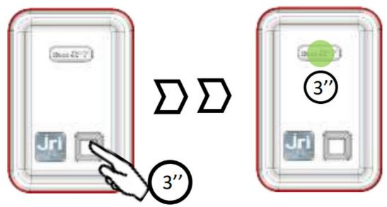
Once activated, the le Nano SPY automatically declares itself in MySirius if it is contact with a Link. It starts to measure and transmit its measurements to My Sirius, at the frequency defined in MySirius, then flashes regularly as a function of its status.
