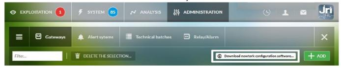
Once the Nano Link is connected to the PC, execute the application « ConfigLink Network.exe » and follow the indications on the screen.
