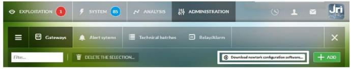
Once the Nano Link is connected to the PC, execute the application « ConfigLink Network.exe » and follow the
