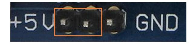
• However, if you want to supply an external power source, you can install it on the two right pins, marked in the following picture:
