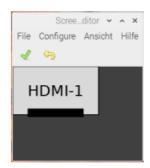
In this window, simply go to Configure > Screens > HDMI-1 > Rotation and select the desired orientation that you want to use for your display.
