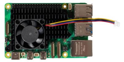
Now mount it from the underside of your Raspberry Pi using the two enclosed screws and washers.
