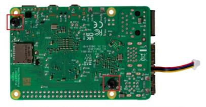
Now insert the fan cable into the fan connection of your Raspberry Pi.
