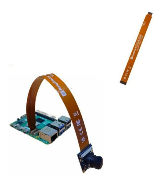
If you want to use the camera module on a Raspberry Pi 5, you must push the clip holding the ribbon cable to the end in the direction of the arrows to remove the ribbon cable already connected to the camera module as shown in the picture below.
