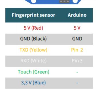
The pin Touch is an output pin, which sends a signal, if a finger has been placed on the sensor.
