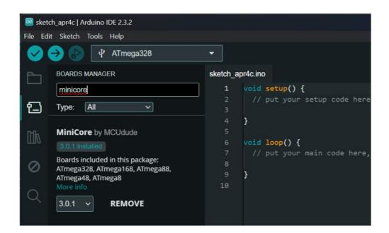
Now select the appropriate board: Tools  $\rightarrow$  Board  $\rightarrow$  Minicore  $\rightarrow$  ATmega328 At Tools  $\rightarrow$  Port, select the port to which your device is connected. At Tools  $\rightarrow$  Variant, select 328PB. And at Tools  $\rightarrow$  Programmer select AVRISP mkll
