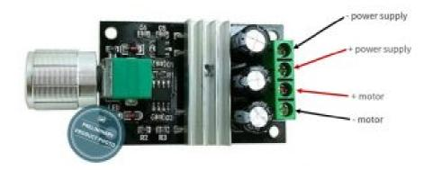
By turning the potentiometer, the speed of the motor is adjusted by PWM.
