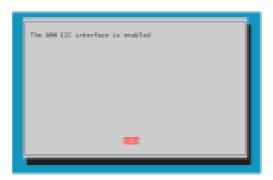
You have now successfully activated I2C. The analog-digital converter is now accessible under the I2C address 0x48.
