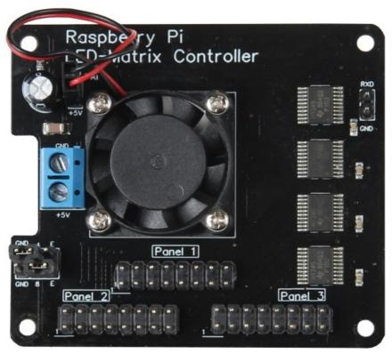
First plug the matrix controller board onto the GPIO bar of your Raspberry Pi. Connect the HUB75 connectors of your matrices with the corresponding connectors (panel 1, panel 2, panel 3) on the controller board.
