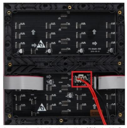
Up to three matrices can be operated parallel while using the 40-pin GPIO strip of the Raspberry Pi. Additional matrices can be connected in series to each matrix. Please make sure to adjust your power supply accordingly. Therefore use the HUB75 connector contact marked with ININ on the matrix.
