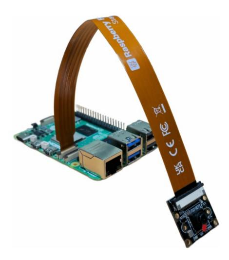
If you want to use the camera module on a Raspberry Pi 5, you must push the clip holding the ribbon cable to the end in the direction of the arrows to remove the ribbon cable already connected to the camera module as shown in the picture below.
