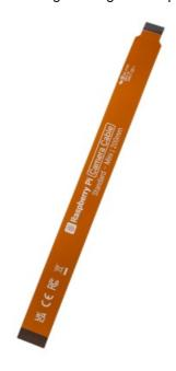
Pay attention to the orientation of the cable, on the camera module the wide black section of the cable must point upwards, while the thin black section on the Raspberry Pi 5 must point towards the clip. The connection via the CSI interface is sufficient, so no further connection is required.
