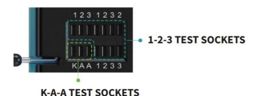
The connectors with identical labeling are connected to each other. Secure your component after you have inserted it by flipping the locking lever at the left of the test sockets.
