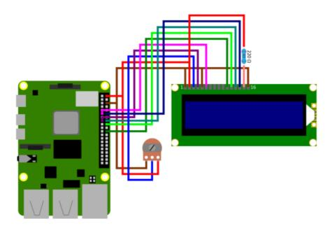
Since the display works with a 5V logic level, you must use a logic level converter if you want to read data from the display with the Raspberry Pi. In this example, the display is only written to, so the Raspberry Pi can be connected directly to the display.
