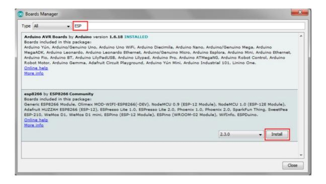
Once you have successfully installed the board, you can select the Gene-ric ESP8266 Module from the list of available boards.
