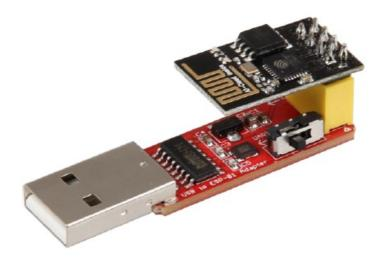
To use the ESP-01S relay module, you must first program the ESP-01S supplied on the product. For this, we recommend programming the ESP-01S with the ESP8266 PROG from 3. First, the Arduino development environment must be prepared for use with the ESP8266. To do this, the following URL is entered in the global settings of the pro-gram as an additional board administrator URL:
