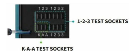
The connectors with identical labeling are connected to each other. Secure your component after you have inserted it by flipping the locking lever at the left of the test sockets.
