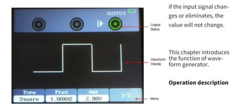
Press the power button to turn on, and then press the "AWG" button to enter the waveform generator function interface.
