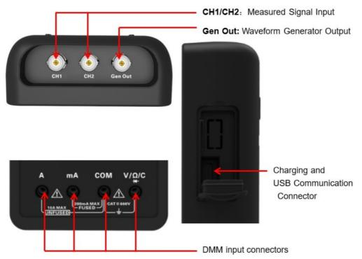
**Gen Out:** The Gen Out terminal of the oscilloscope without signal generator function always outputs 2V @ 1KHz square wave.
