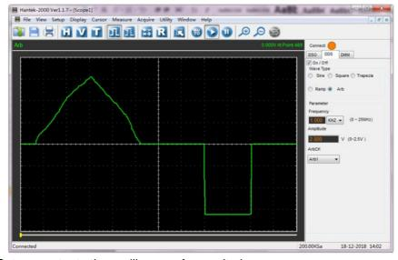
12. Connect the Gen Out connector to the oscilloscope for monitoring
