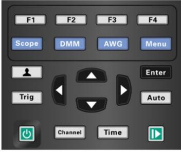
In generator, press the button to confirm after entering the character.
