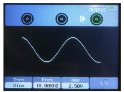
Second, press F1 button to open the digital keyboard again, use the up, down, left, right direction keys and "Enter" key to set offset parameter, select "OK" and press Enter button to confirm.
