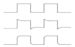
3. If necessary, use a nonmetallic screwdriver to adjust the variable capacity of your probe until the shape of the waveform turns to be the same as the above figure. Repeat this step as necessary. See the figure below for the
