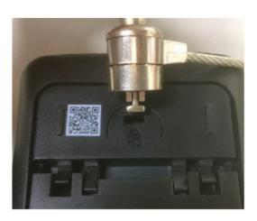
A safety keyhole is reserved on the back shell of the oscilloscope. Users need to purchase the safety lock by themselves. Wrap one end of the safety lock around a hard-to-move object, insert the other end into the safety lock hole, turn the key clockwise to lock the instrument, and then pull out the key. In this way, the most basic anti-theft requirements can be achieved.
