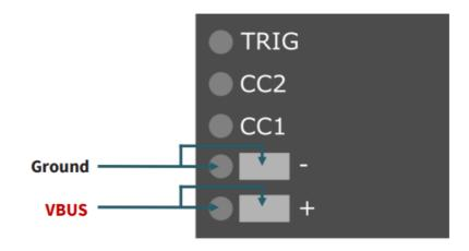
The trigger pin on the board has the same function as the button. By set-ting the pin LOW, pressing the button is simulated.
