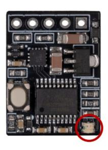
To set the modes as default, first plug the board into your power supply while holding down the button on the board. Now the LED will start flashing colourfully. Now you can select the desired mode using the button. Now press and hold the button to confirm your selection. Finally, disconnect the power supply from the module and then reconnect it so that the module now starts directly in this mode.
