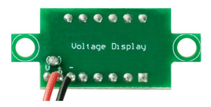
You can also measure voltages below 3 V with this voltmeter, but for this you have to supply power to the display regardless of the measuring voltage. This requires soldering, because you have to remove a solder bridge on the back of the unit and solder more wires to the board.
