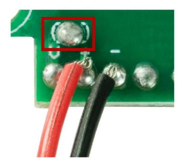
Now you have a new pin assignment on the measuring device. Please note that two ground connections must be connected to the negative terminal of the measuring device (black cable) (one for the measuring voltage and one for the supply voltage).
