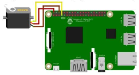
Since the motor is connected, you can transmit the following code examples to your Raspberry Pi and test their functions.
