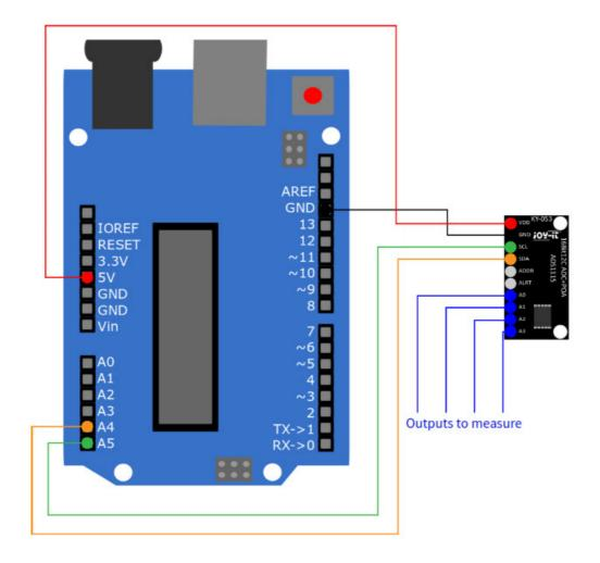
Here, the analog-digital converter is connected to 5 V. So the converter can only measure 5 V on the analog inputs without suffering permanent damage.
