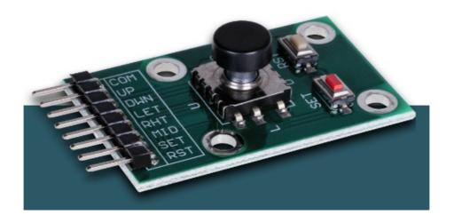
Navigation switch with 5 directions and two additional buttons
