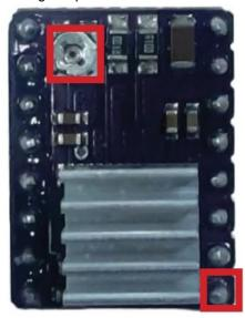
Once the current has been adjusted according to the motor specification, the motor can be connected and tested. During operation, it should be checked that the motor rotates smoothly, that no excessive heat is generated and that the driver does not go into overload protection. If the motor gets too hot or behaves unusually, the setting can be fine-tuned again.
