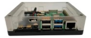
6. Therefore, place the large board on the GPIO bar of the Raspberry Pi. The circuit board is inserted at a slight angle so that the connections fit easily into the panel. Important: Should you use the audio cable, care must be taken to ensure that the cable does not get under the jumper pins on the bottom, otherwise the top PCB will not mount correctly.
