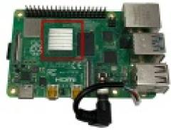
3. Afterward, connect the small board to the two micro HDMI connectors. Optionally, you can now connect the cable from the AUX connector to the appropriate socket on the circuit board. The cable should lie as flat as possible against the board, otherwise, space problems may occur.
