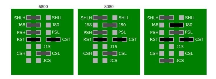
The components marked in black (marked with X in the table) are Don't Care components. This means that it does not matter, where these components are set.
