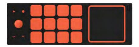
The Play Drum Pad is composed of 12 identical pads, each of them has its own percussive sound. Select a drum kit from the app and discover the 12 associated sounds of each kit.
