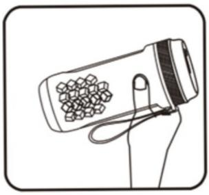
4. Double click the start button switch diagonally downwards by about 45 °, and the work indicator light will display in blue. The product will work for a cycle of 30 seconds.
