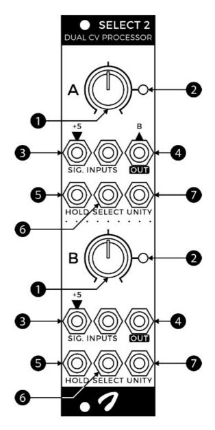
both CV and audio. However, the exceptionally low leakage rate also allows minutes-long storage of pitch-accurate CVs. All of Select 2's gate inputs are uniquely designed to be driven reliably even from weak, slow, bipolar signals. They feature Schmitt action, with a +2 V low and +3 V high logic threshold.
