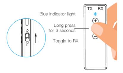
If there is no device access after turning on, the transceiver will automatically shut down in 5 minutes.
