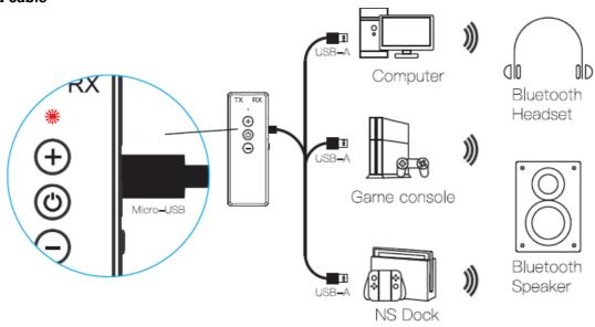
Plug one end of the data cable into the charg-ng rt of the transceiver, the other end into PC, PS4, Switch dock, and other devices that support USB audio output. (Some USB rts only support oharg-ng, Not for audio transmission.)
