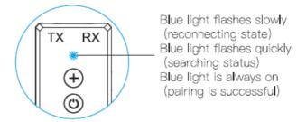
After power on, the transceiver will automatically connect to the last connected device. If the connection is unsuccessful, it Will enter the searching status.
