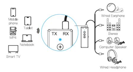
Plug the 3.5mm audio cable of the wired headset or wired speaker into the audio Interface (marked RX) on the Bluetooth transceiver
