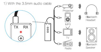
Plug one end of the 3.5mm audio cable into the audio interface {marked TX) on the transceiver, and the other end into the AUX interface on the TV or other equ-pment
