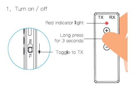
If there Is no device access after turning on, the transceiver will automatically shut down In 5 minutes.
