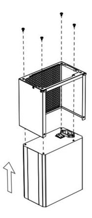
**Note:** The power plugs need to be inserted into the power supply first, and then installed on the front panel.
