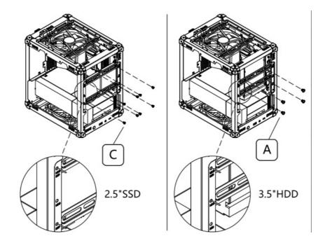
2.5" SSD or 3.5" HDD install on the multi-functional brackets, and than mount on the corresponding mounting points
