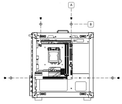
The motherboard is placed into the chassis and locked with screws.
