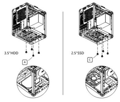
The hard disk is installed on the bottom plate, and the mounting holes are locked with screws. The 3.5HDD hard drive and fan share the same installation location.
