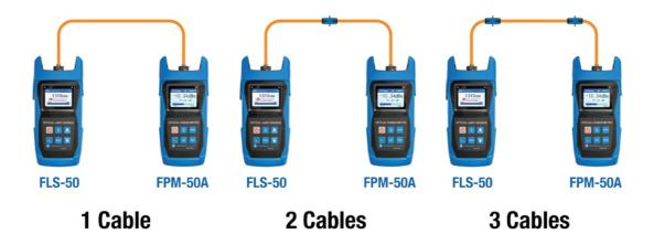
\*Note for multimode testing, the use of a mandrel wrap ring is recommended to use for the test cable plugged into the optical light source.
