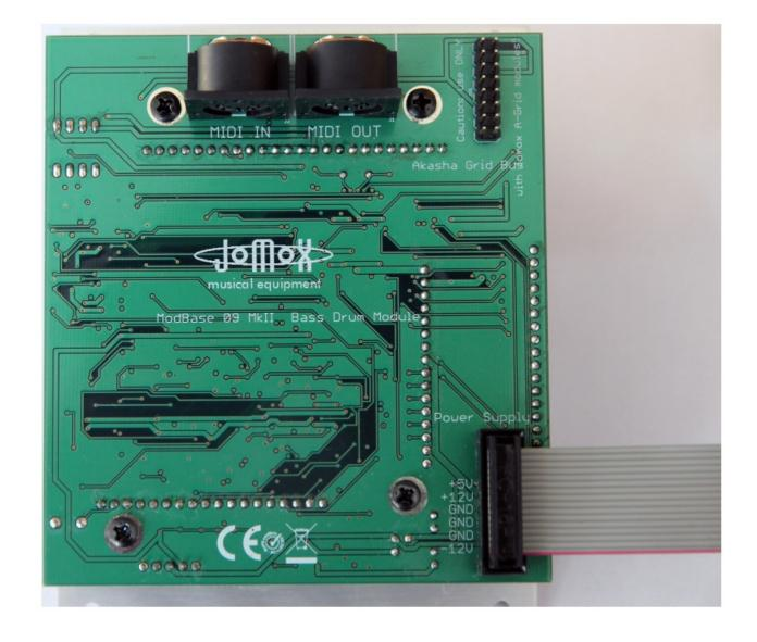
Don't flip the cable but connect it as shown on the picture.
