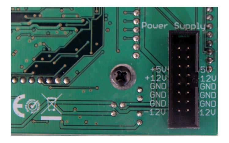
Connect the other end of the ribbon cable to the module as shown on the picture. The cables are fairly short which is good in electrical means to the relatively high power consumption of the module.
