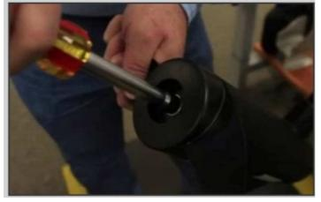
**NOTICE**: Over tightening the nyloc nut will start to bend the prop pin and cause the prop hub to rub on the drive's lower case.
