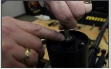
8. Tighten the nyloc nut until the prop shaft is even with the top of the nyloc nut.
