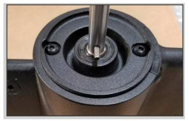
7. Before putting nyloc nut on the shaft, lightly spread anti-seize compound on the prop shaft threads. This compound will help prevent small slivers from jamming in the threads that prevent motion in either direction.
