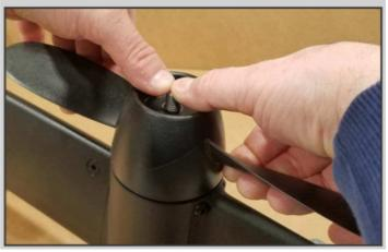
4. Remove the prop pin from the prop shaft.
