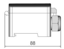
In order to reach IP 65 protection according to EN 60527, the cover has to be bolted e.g. using a screw 3,5×10 mm according to EN 7981.
