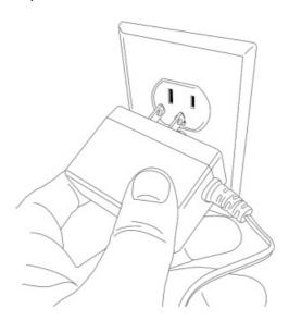
Plug the barrel jack of the power supply into the "DC-IN" port on IQ WiFi 6. Plug the power supply into the wall outlet.
