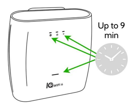
IQ WiFi 6 will automatically power up, configure as the primary IQ WiFi 6, and download any needed updates. The LEDs will be solid green when complete\*. (Up to 9 min)
