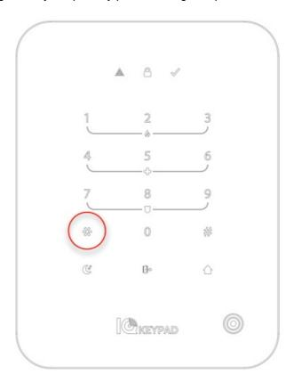
NOTE: The IQ Keypad may also be manually paired to a panel by using the sensor ID printed on the device beginning with 372-XXXX. If manual learn is used instead of Auto Learn, you must network the device after pairing is complete by pressing and holding [\*] for 3 seconds.
