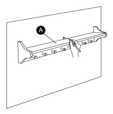
Step 5 Insert the wall plug (C). Hang the hook rack (A) and screw the screw (D) through the metal plate.
