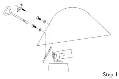
Place the shade over the table lamp and align the holes in the shade with the holes in the lamp plate. Secure the shade by fitting the protective washers to the screws and then tighten the screws using the screwdriver provided. If cross threading occurs, undo and start again. Take care not to overtighten as this may cause damage to the fitting.
