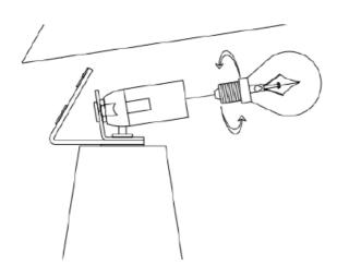
Fit the bulb, type and wattage as indicated on the fitting (bulb not supplied). The wattage indicated must not be exceeded.
