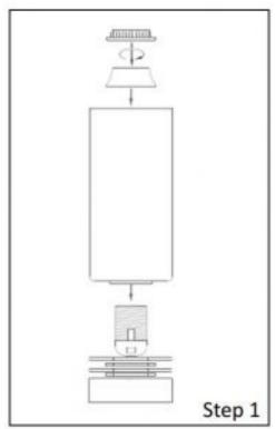
Remove the shade ring already attached to the lamp holder section. Carefully place the shade glass followed by the spacer (widest end first) over the lamp holder. Secure the assembly in place by refitting the shade ring removed earlier. Take care not to over tighten as this may cause damage to the fitting. Ensure all components are straight and aligned during this assembly process.
