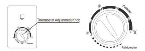
The inside temperature of the freezer is regulated by a thermostat adjustment knob.
