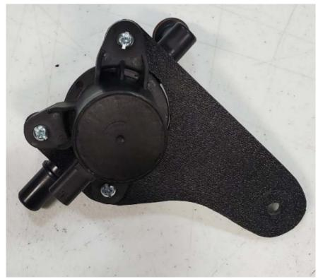
4. Slide the brown O ring up and out of the channel it's sitting in and use oil or any lubricant to install the supplied 3/4" PCV hose on to the fitting on the bottom of the solenoid.
