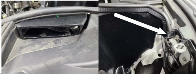
7. Lower air filter down into the airbox first, then with the silicone reducer on the tube with clamps loose, connect
