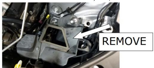
4. Remove the IAT sensor (twist lock) from the stock inlet tube and PCV fitting(2018 only). Use the JLT supplied gasket, screws and IAT sensor pad to assemble the JLT tube.
