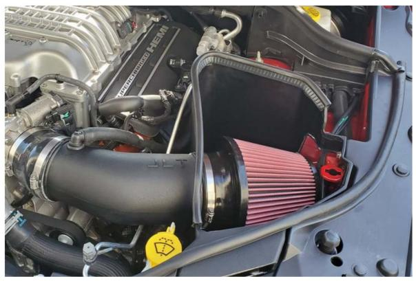
Oil Filter: The frequency you should clean your filter will depend on your driving conditions. It is recommended to check your filter at every oil change or 3,000 miles. If there is a buildup of dirt as thick as the wire mesh, then it's time to clean your filter.
