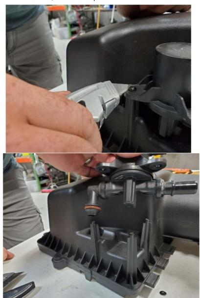
3. Use the supplied hardware and bracket to mount the solenoid to the bracket as shown.
